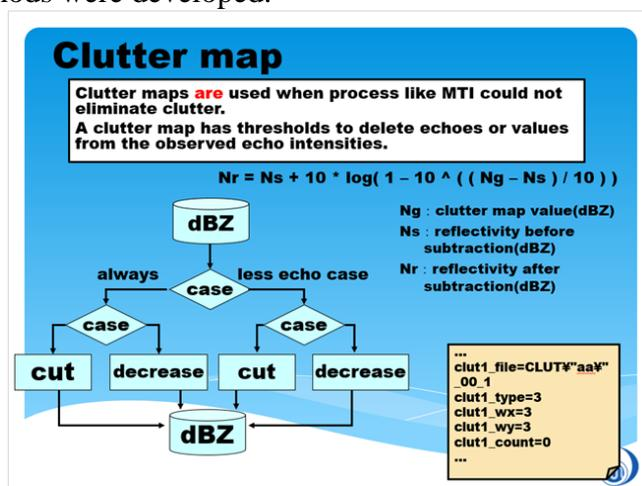
**Figure 10.** The process flow diagram of the clutter map.
