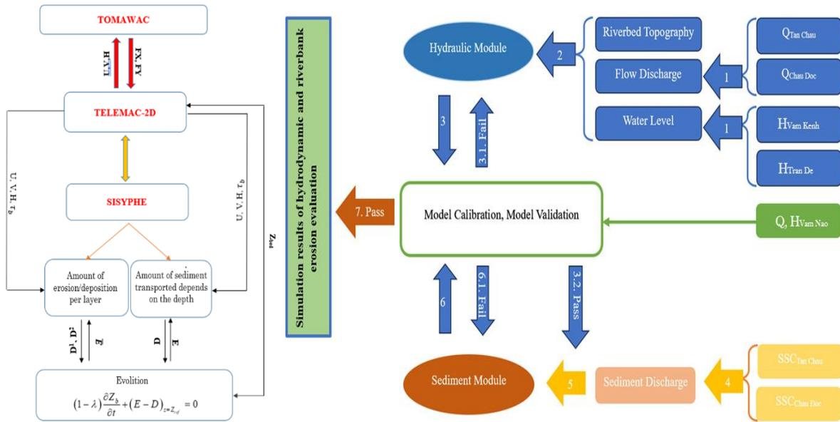
Figure 1. General flowchart of study using TELEMAC model.
