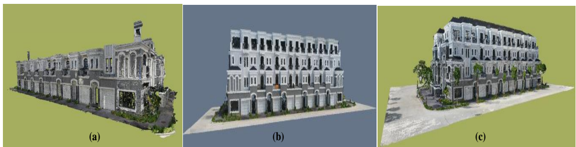
Figure 14. Neighboring villa’s TC point cloud after noise filtering (a), Neighboring villa’s UAV point cloud after noise filtering (b), Neighboring villa’s UAV and TC point cloud after precision matching (c).
