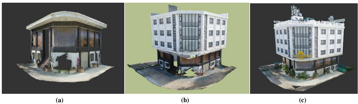
Figure 13. Independent building’s TC point cloud after noise filtering (a), Independent building’s UAV point cloud after noise filtering (b), Independent building’s UAV and TC point cloud after precision matching (c).
