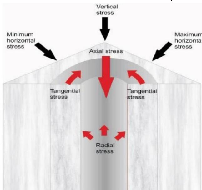
**Figure 2.** In-situ stress model around a drilled wellbore
