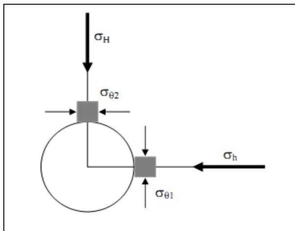
**Figure 4.** Tangential stress at the wellbore wall [5].
