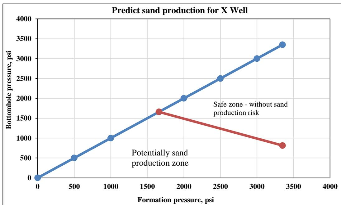
**Figure 5.** Critical drawdown pressure results for well X.
