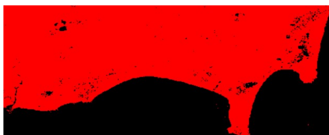
Figure 5. Result of applying the threshold for separation between land (red) and water (black).
